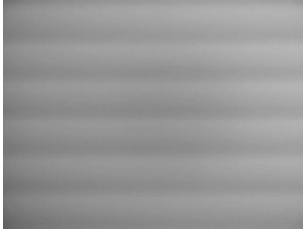
Figure 11: Flicker in image of white uniform object illuminated by strong fluorescent light
